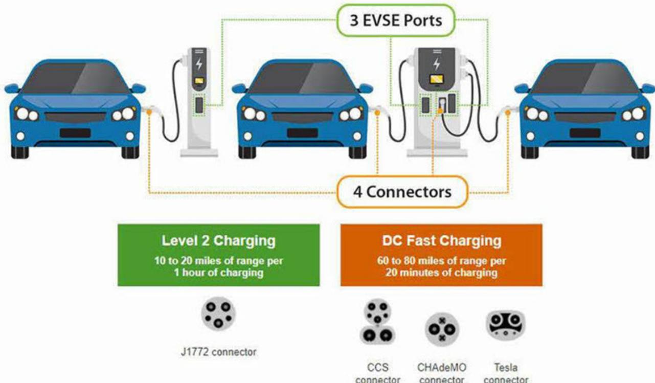
**Note:** CCS = Combined Charging System; EVSE = electric vehicle supply equipment. Source: US Department of Energy
