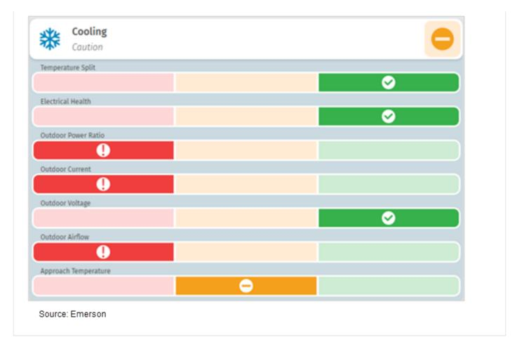
Implementing FDD could help relieve headaches associated with HVAC issues and repair. Customers can share the diagnostics with their contractor, cutting down assessment time and delay in getting the customer's system back on track and operating efficiently.
